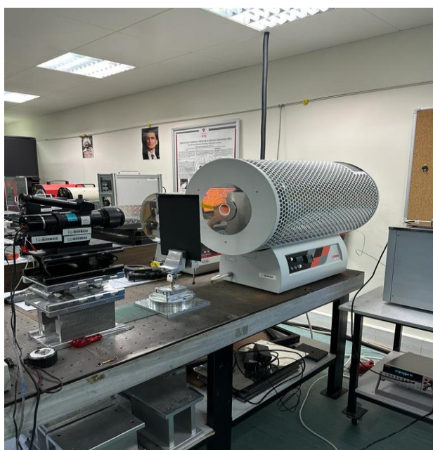
Fig 2: Calibration at high temperature using high emissivity blackbody.
