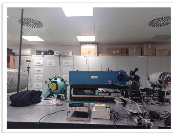
Fig 6: Monochromator used for spectral responsivity measurement.
